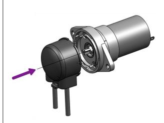
2.Clockwise rotation 15° slot in place Rotor rotation is recommended clockwise, The orientation of the entrances and exits is shown below
